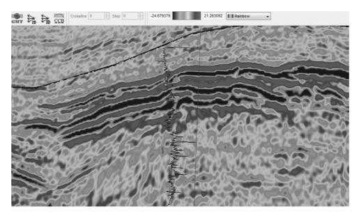
Fig. 10. 1569 line colored inversion profile of LW3-1-1
