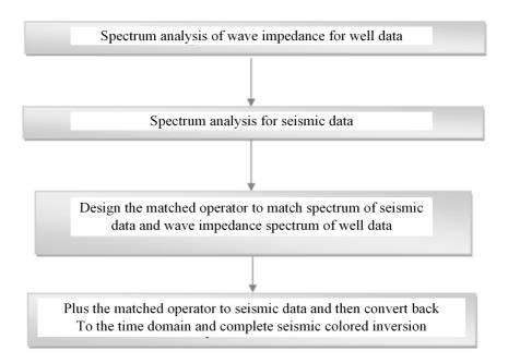
Fig. 8. Process of color inversion
